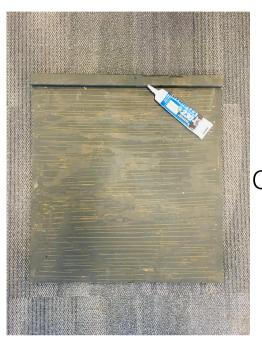
1. Put the bigger board down first. Set it where you are most comfortable to use caulking and a drill. Lay a strip of caulking and place the long, thin piece on the top edge and push down.
