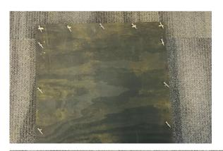
**5.** Line up the holes on the back side and attach the back with screws in
